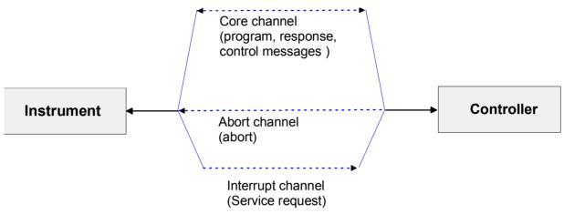
Fig. 5-3 VXI-11 channels between instrument and controller
