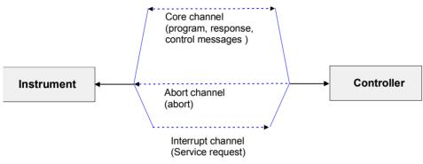
Fig. 8-3 VXI-11 channels between instrument and controller
