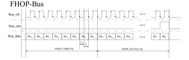
Input control signals for FHOP on the serial FHOP bus (BERT BNC connectors)
