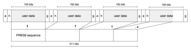
Fig. 4-5 TDMA signal generated by the **WinIQSIM2** software with user data that contains the PRBS data sequence. The PRBS sequence is continuously written to the user data fields.
