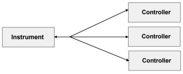
Fig. 8-4 Remote control via LAN from several controllers
