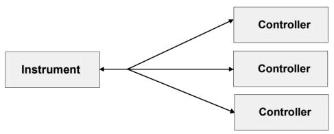
Fig. 5-4 Remote control via LAN from several controllers
