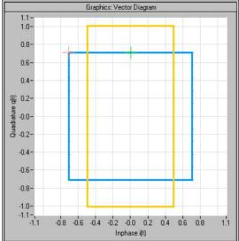
Entering a gain for the Q signal means that the Q vector is amplified more than the I vector by the Q path of the input amplifier.
