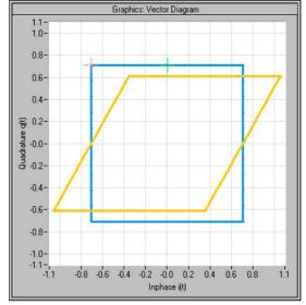
A negative error means a phase angle less than 90 degrees:
