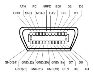
Figure 8-1 Pin assignment of IEC/IEEE-Bus interface
