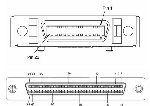
Fig. 8-5 Pin Assignment of Port 1 and Port 2
