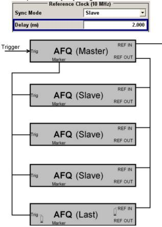
*Fig. 4-1 Connection of several R&S AFQs for precise synchronization* The parameters for the synchronization are set in the Reference Clock area of the Clock dialog.
