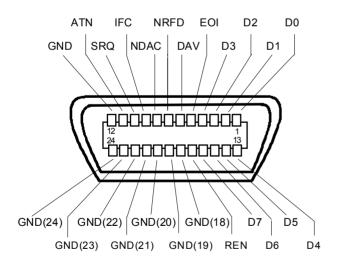
Figure 5-1 Pin assignment of IEC/IEEE-Bus interface
