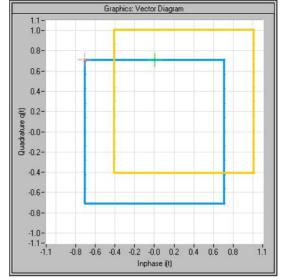
Effect of an identical offsets for both signal components:
