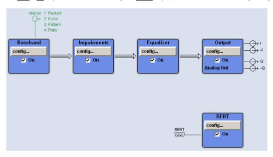
Each block represents a function of signal generation. The function is indicated in the headline of the block, e.g. **Baseband.** In this block, the arbitrary waveform generation is set, for instance.
